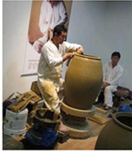
Making flat bottom first and building the wall with coils (kwon sang technique)
