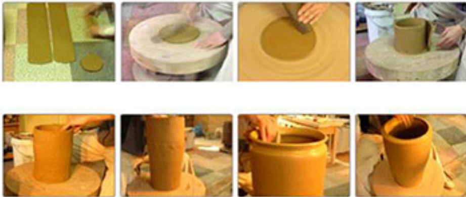
Building the wall with slab on the bottom (Chaebaqui technique, Yunjuk technique)
