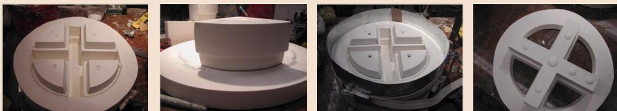
*Left: Making the gang mould. Left centre: Hydrostone model on set up slab. Right centre: Preparing to cast gang mold spare. Right: Gang mold spare.*
