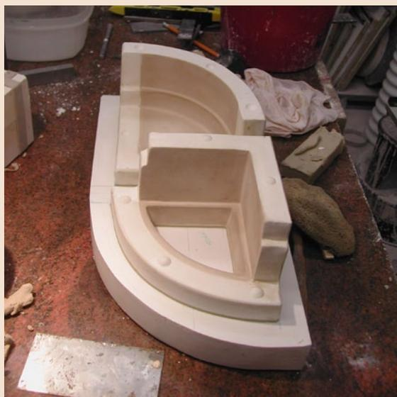
*Top left: Set up to pour rubber mould of the quadrant from Ren-Shape model. Top centre: Set up to pour rubber mould of the quadrant from Ren-Shape model.*
