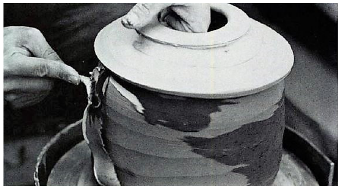
Les Manning. Wet trimming the surface clay exposes clay colour and pattern. Ceramics Monthly, June 1982.
