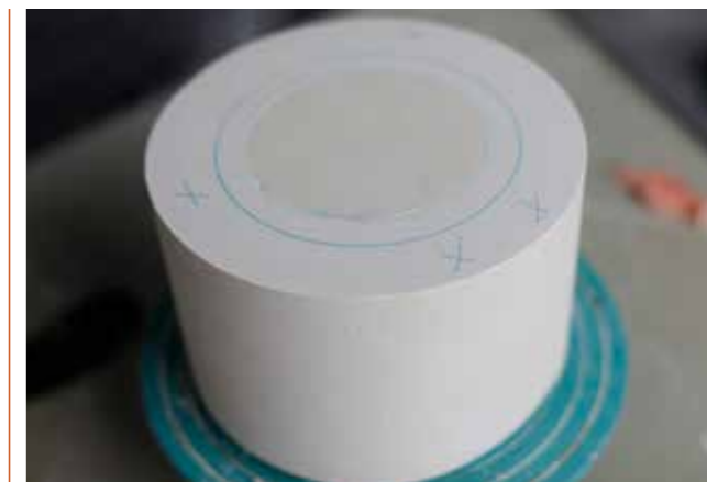
22 I plot the position on top of the mould for the location points/natches for the reservoir ring and spare.
