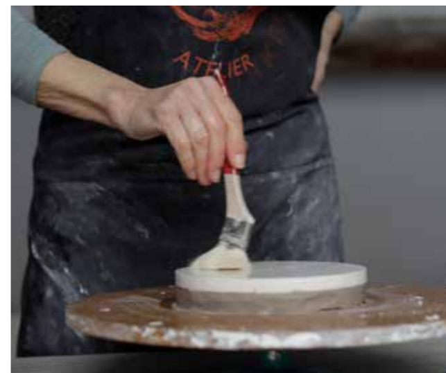
9 I soft-soap, or 'size', the moulding batt three times as this acts as a barrier between the two layers of plaster. This will help release the mould later; if you don't use soft-soap they will stick together. I add the soap with a brush, then use a damp sponge to remove the excess.
