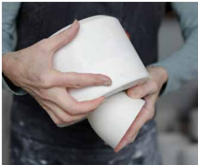
29 As soon as the plaster is set, or cured, I remove the model, spare and reservoir ring from the mould.
