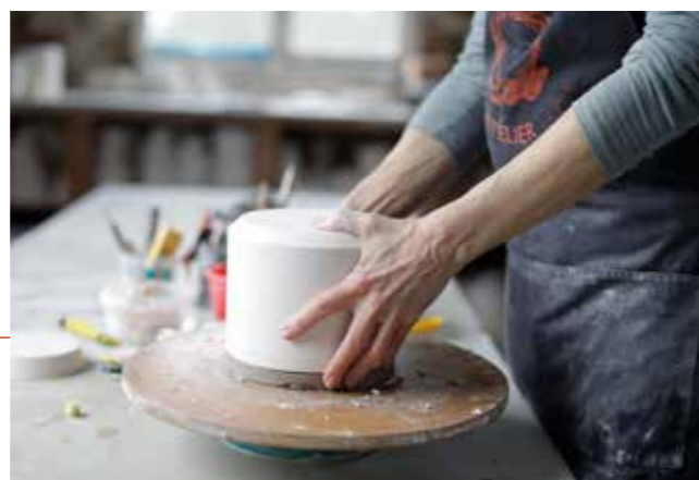
18 Once set, I remove the cottle. I then bevel the edges using a metal kidney to soften or remove sharp edges.
