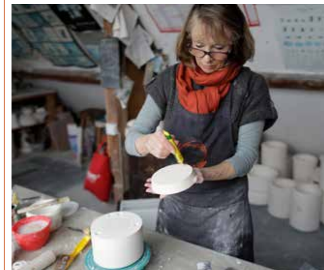
26 Three dots of UHU glue are used to secure the spare in position, following the pencil-marked guidelines.
