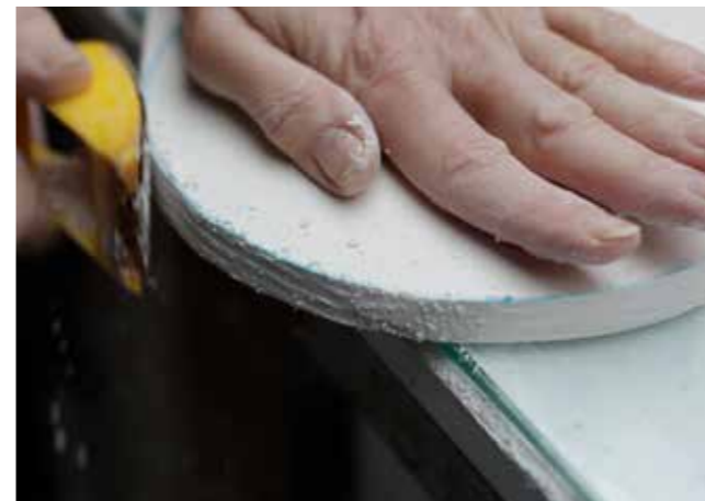
6 I use a surface-forming tool called a Surform to make the moulding batt as circular as possible.
