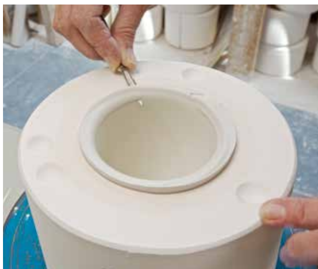
32 I cut off the 'spare', or surplus slip, with a scalpel or sharp cutter to reveal the rim.
