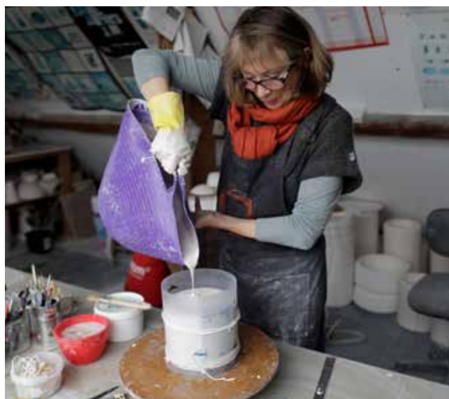
17 I pour the plaster into the cottle and leave it to set, or cure. In the case of the plaster I use, this takes approx. 5 minutes.
