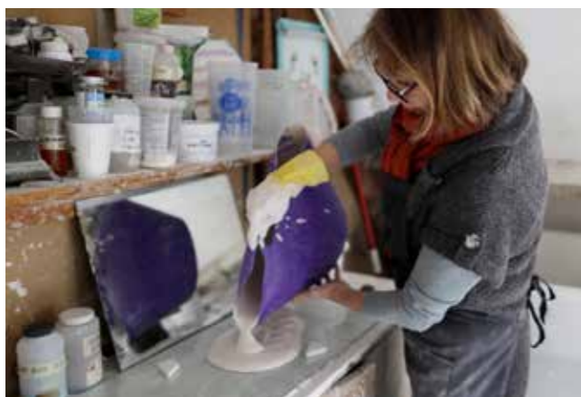
3 I then pour plaster onto a sheet of glass to make a moulding batt. This is a flat piece of plaster, cut to size, that determines the size and diameter of the mould.
