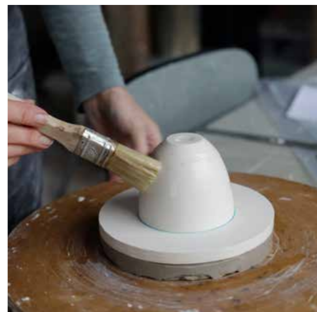
11 The model is then soft-soaped three times and the whole thing is buffed with a dry brush.
