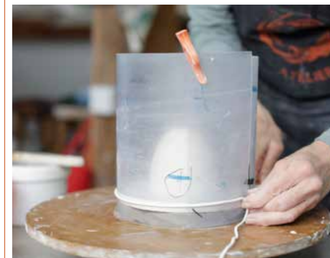
12 The next step is to place 'cottling' plastic around the model and batt, securing it in place with a peg and string. Cottling plastic is a flexible sheet of plastic that is used to create a retaining wall around the mould to hold the plaster in place while it sets.
