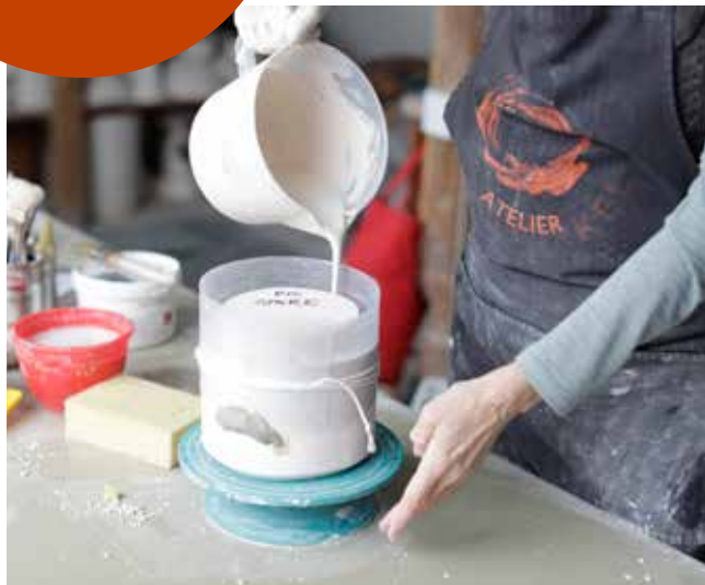
27 Cottling plastic is placed around the top of the mould and plaster is poured between the spare and the cottle.
