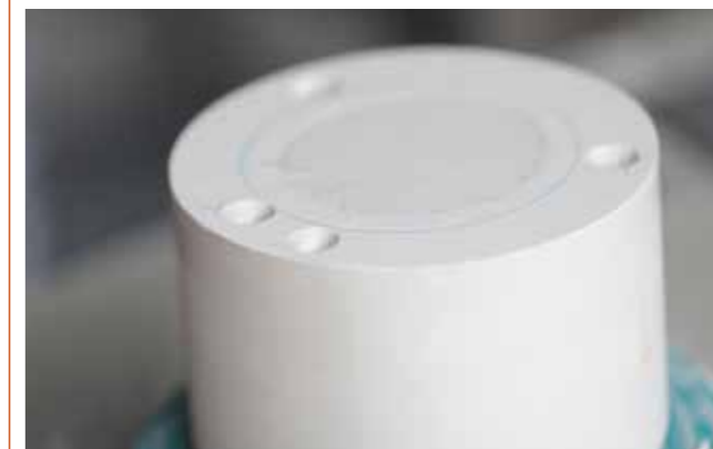
24 This is the top of the mould with the natches in place.
