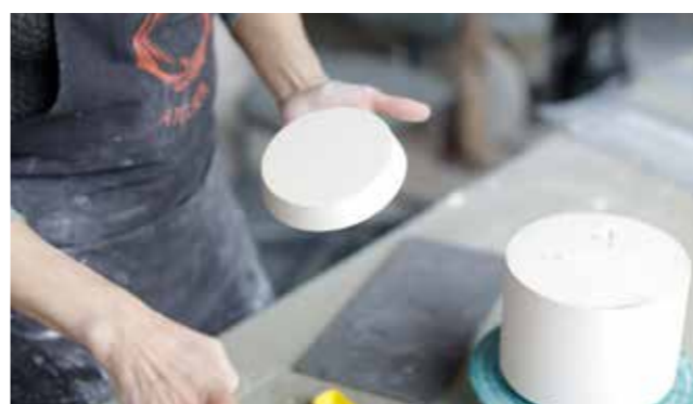
21 I then soft-soap the spare, which is a turned plaster disc that is 2cm larger than the diameter of the model.
