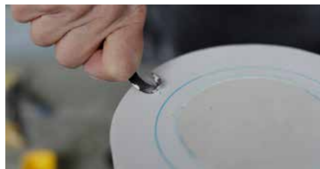
23 The natches are made using a forged steel tool, or sometimes I use a half penny coin to gauge the size.
