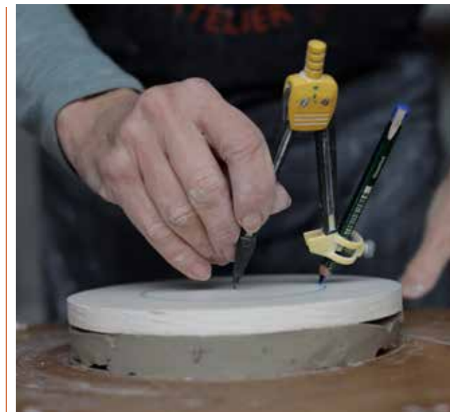
8 The moulding batt is then raised up with clay by around 2cm to make securing it easier and to prevent slipping. The diameter of the model is then plotted onto the moulding batt using an indelible blue pencil and a compass.
