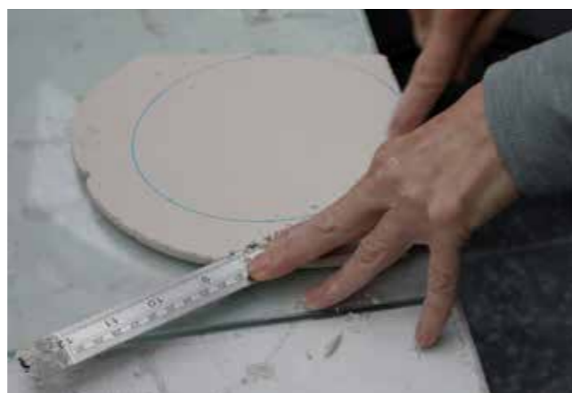
5 Once the plaster is set, the moulding batt is cut out and trimmed to size. The total size is the diameter of the model plus eight centimetres.
