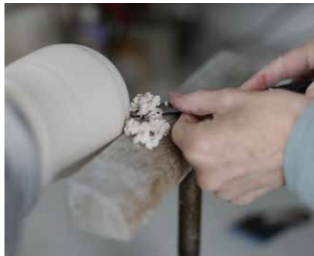
2 I create the model by turning it on a lathe, using a chisel to shape the plaster into the desired form. If you don't have a lathe, the model can be made out of clay, either thrown or handbuilt, and this can be used to create the plaster mould.
