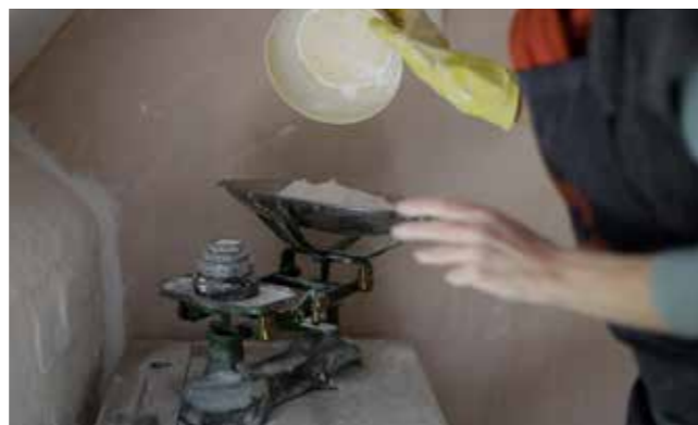
14 For the first part of the mould, I measure the water and powdered plaster: one pint of water to one and three-quarter pounds of plaster. In this instance I'm using Newcast 96 plaster.
