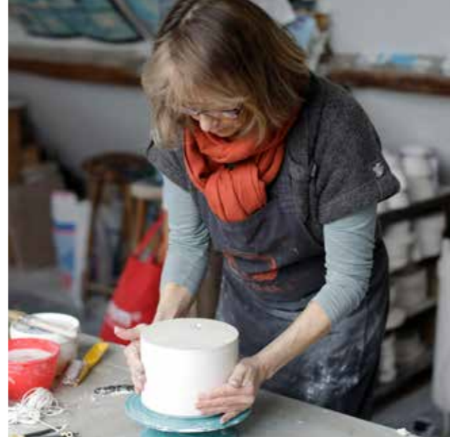
20 The mould is turned the right way up in preparation for the creation of the reservoir ring. This is a separate removable ring of plaster that acts as a reservoir for the casting slip on the top of the mould. It also allows for variable casting thicknesses, which is indispensable for multi-layered casting and neat rims.
