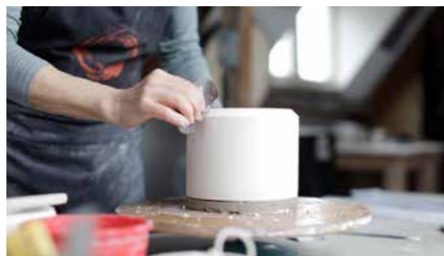
18 Once set, I remove the cottle. I then bevel the edges using a metal kidney to soften or remove sharp edges.
