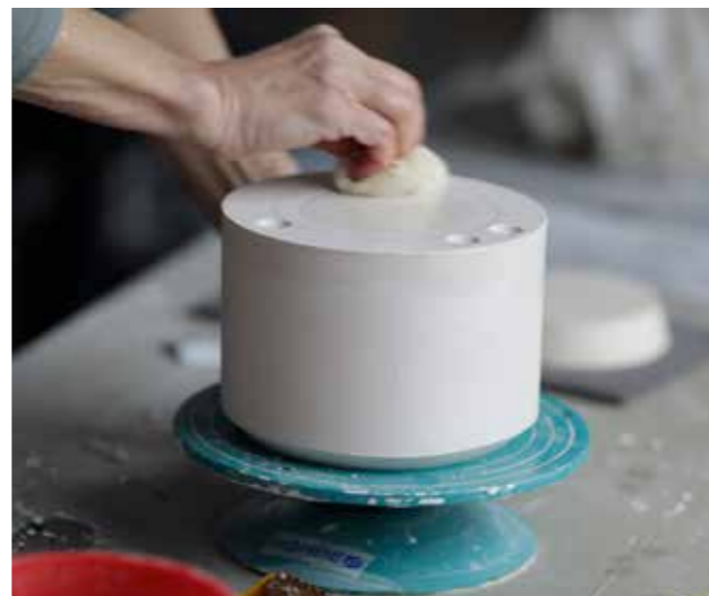
25 The top of mould is then soft-soaped.
