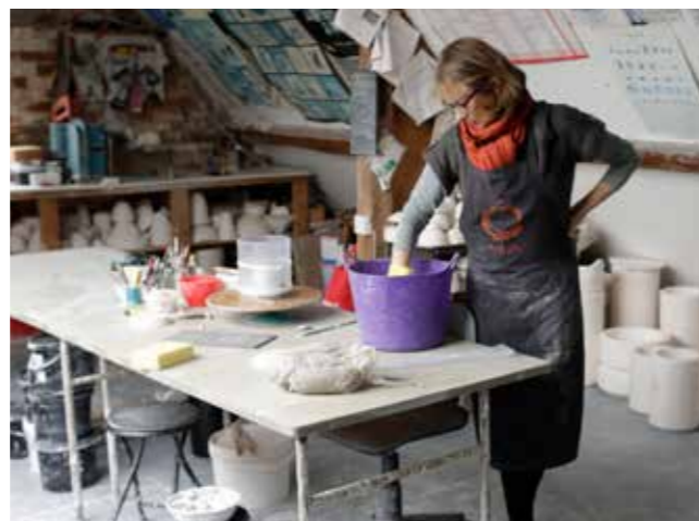
16 I mix/blend the plaster for around 15–20 minutes.
