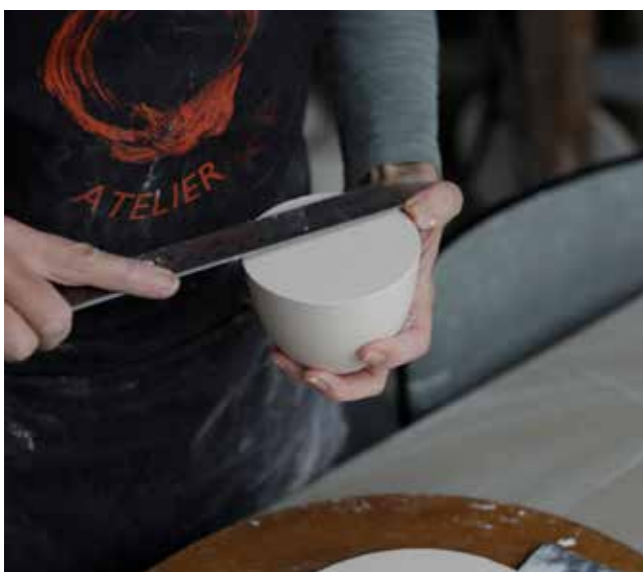
7 I measure the diameter of the model accurately in order to ensure the mould is the correct size.
