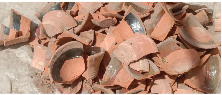
After baking process when we got from the kiln we then crush this glaze with the help of a hammer crusher and then grind it in "Jhaand", a kind of crusher machine.
