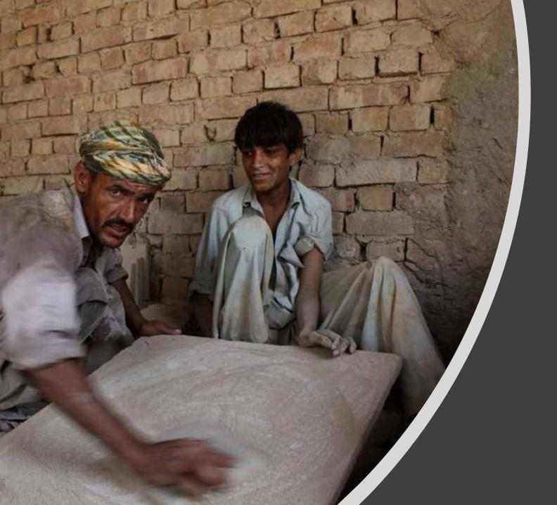
The tiles are sanded on a cement block to make the surface even and prepare for the decorative finish.
