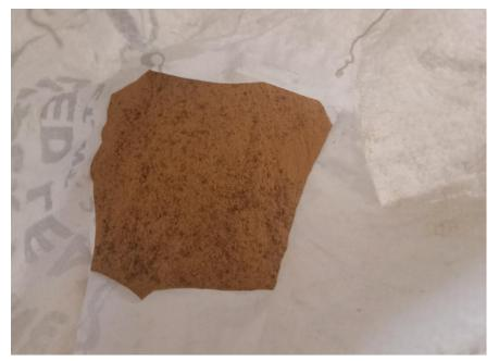
After glaze was ready in powder form we sieve it with 100 mesh screen than apply in liquid form on painted tiles and plain tiles.
