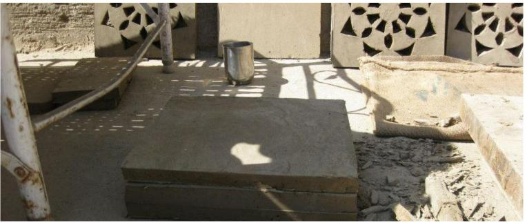
Tiles are placed on a flat, even floor after 24 hours these tiles are harder when completely dry.
