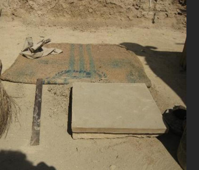
Removal of unwanted dots and sand on front and back area of tile.
