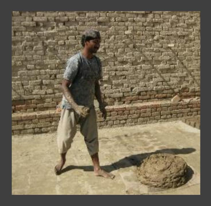
Clay wedging process, clay is thrown rapidly on floor for removing air bubbles from clay.
