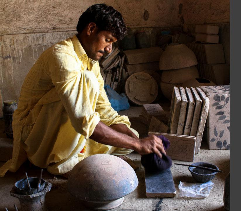
After dry Engobe we start to trace different designs on tracing paper template and then pinhole the outlines with the help of needle, the template which we are calling in our language it's "Khaako".
