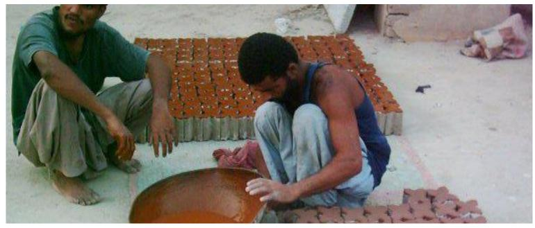
Different glazes applied on tiles and other products in liquid form, we prepared the glaze and mixed the binder and some lead powder for shine.
