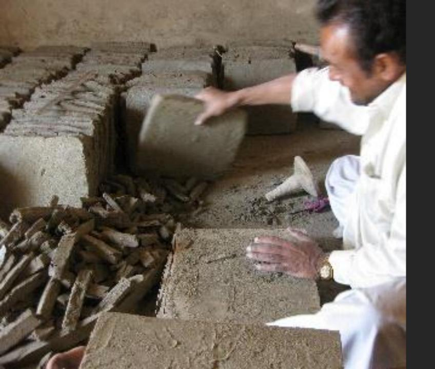
Tiles in leather-hard form are ready for cutting into different sizes.
