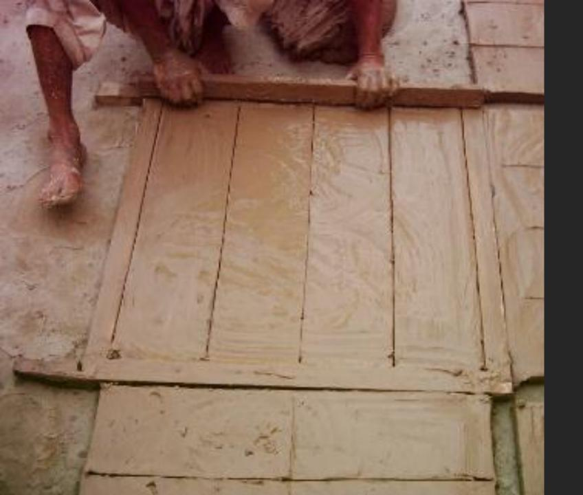
Cutting in order of different sizes during the slab making process.
