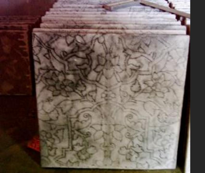
Tracing paper is placed on tile surface edge-to-edge and we apply charcoal powder on the tracing paper for transfer of design on tile surfaces.
