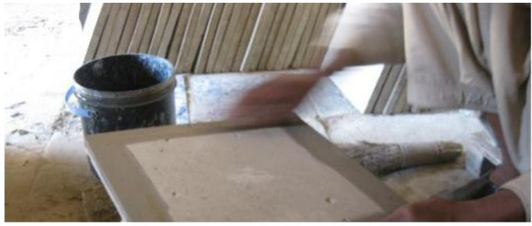
Finishing process of filling edges with clay paste (paste for filling which we made with clay and sand) it is called "Khhaar".
