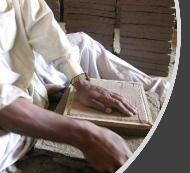
Tiles are cut with different wood-frame stencils which are called "Kaarab", before cutting method we press them again to make an even surface.
