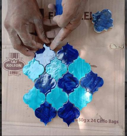
Kacha Rang tile includes color applied to the tile after it is fired in the kiln. This color is not permanent or waterproof. The tile painted with this technique are just for decoration.
