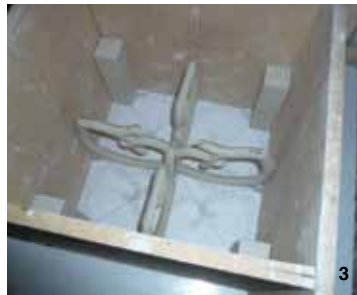
3 Four pieces are placed in a wooden box and joined together vertically at 90° to create the first layer.
