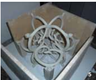
5 After another vertical layer is added and the piece dries, two sides of the box are unscrewed.
