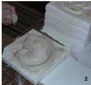
2 Once the molds are drained and the clay is dry enough to release from the plaster, the mold is opened.
