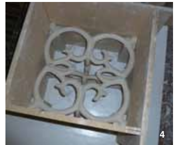
4 Next, four more pieces are joined at right angles to the first layer. The corners are supported by clay posts.
