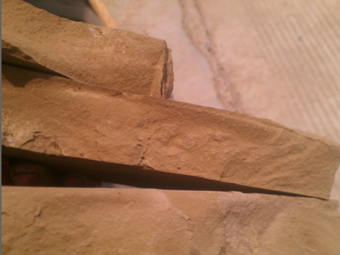
Section of the air-dried adobe before kilning
