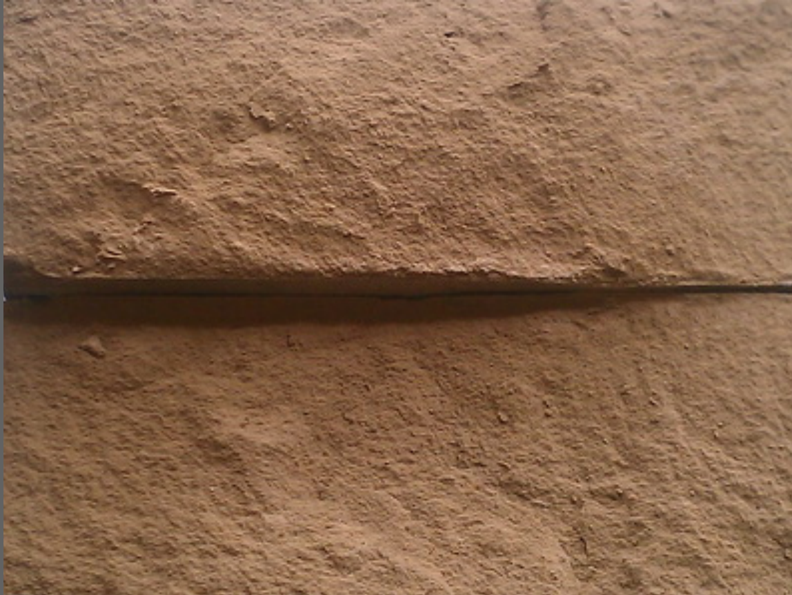
Section of the air-dried adobe before kilning
