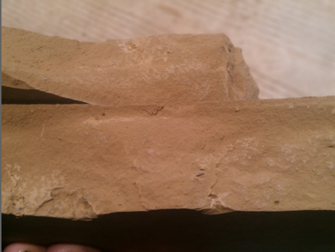
Section of the air-dried adobe before kilning
