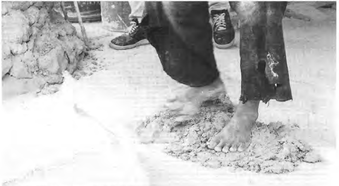
Wedging clay with feet after slaking down and drying by evaporation.
