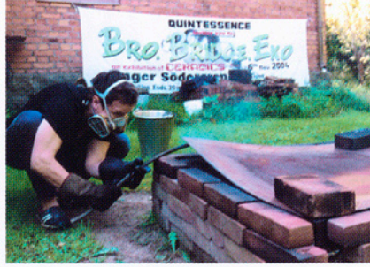
Inger Sodergren controlling the flames by opening and closing the metal lid.
