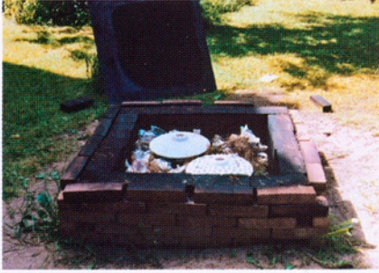
Kiln packed with newspaper and pine. Dishes partly covered with resist clay and turned upside down.
