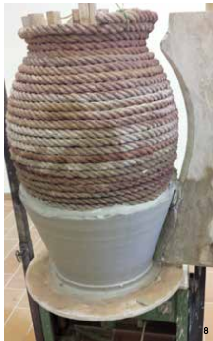
4, 5 Coiling a thick rope around the wooden armature, starting at the slab base of the jar on the wheel head and working toward the top. 6 Once the rope is secured to the armature, the wooden profile template is clamped to the metal armature. 7 Attaching the first coils of clay to the armature and slab base of the jar, smoothing and compressing by hand. 8 After adding coils and compressing by hand, as the wheel turns, the profile template removes excess clay and further smooths and compresses the walls of the jar. 9 A completed coil section, ready to be compressed and shaped by the profile rib.
