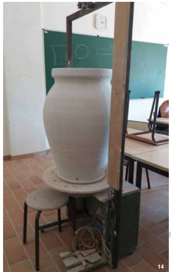
10 Turning the wheel once more at the end of the building process to compress the walls and even out thickness. 11 Using a rubber rib to further compress the surface and remove any air bubbles. 12 Cutting excess clay from the jar's rim using a fettling knife. 13 After removing the pole, armature, and rope, the rope texture can be seen on the inside of the jar. 14 The finished piece is allowed to dry slowly prior to firing.
