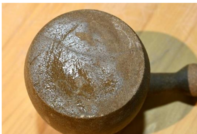
Figure 3. Sintering and water absorption of traditional material experimental quartz sand pottery pots at 1230^{\circ} C
