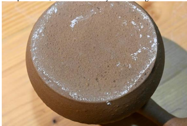
Figure 5. Over burning and foaming of Dongguan black mud, white mud and quartz sand pots at 1280° C
