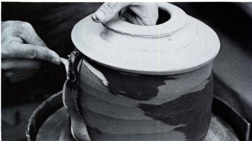
Preparing to throw a multicolored object, Les paddles wedged lumps of porcelain and stoneware into a uniform shape.
