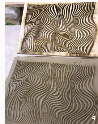
3 An example of a custom pattern design, laser cut using a thin plywood board. 4 The custom-designed laser-cut wood board is carefully pressed onto a slab to create an embossed effect. 5 A 3D-printed shape with thin walls is pressed downward to cut its shape out of a slab of clay.
