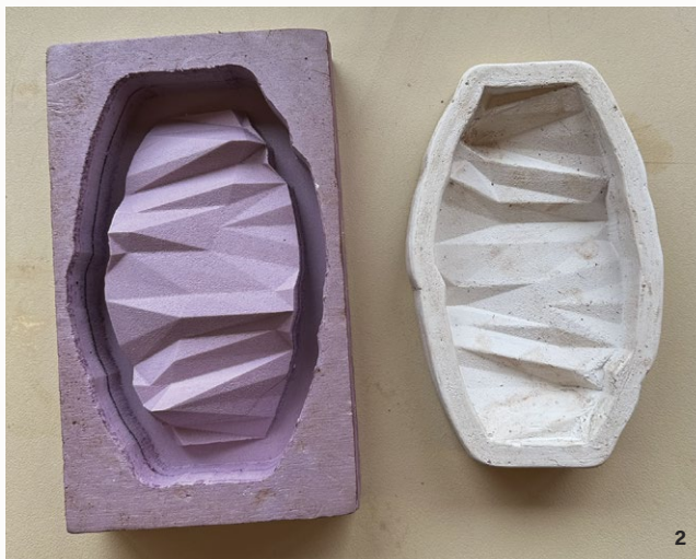
1 A CNC milling machine cutting a block of foam. 2 An example of a completed CNC-milled foam block (left) and the plaster mold that was cast into it (right).
