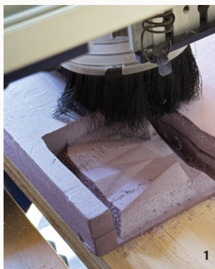
1 A CNC milling machine cutting a block of foam. 2 An example of a completed CNC-milled foam block (left) and the plaster mold that was cast into it (right).
