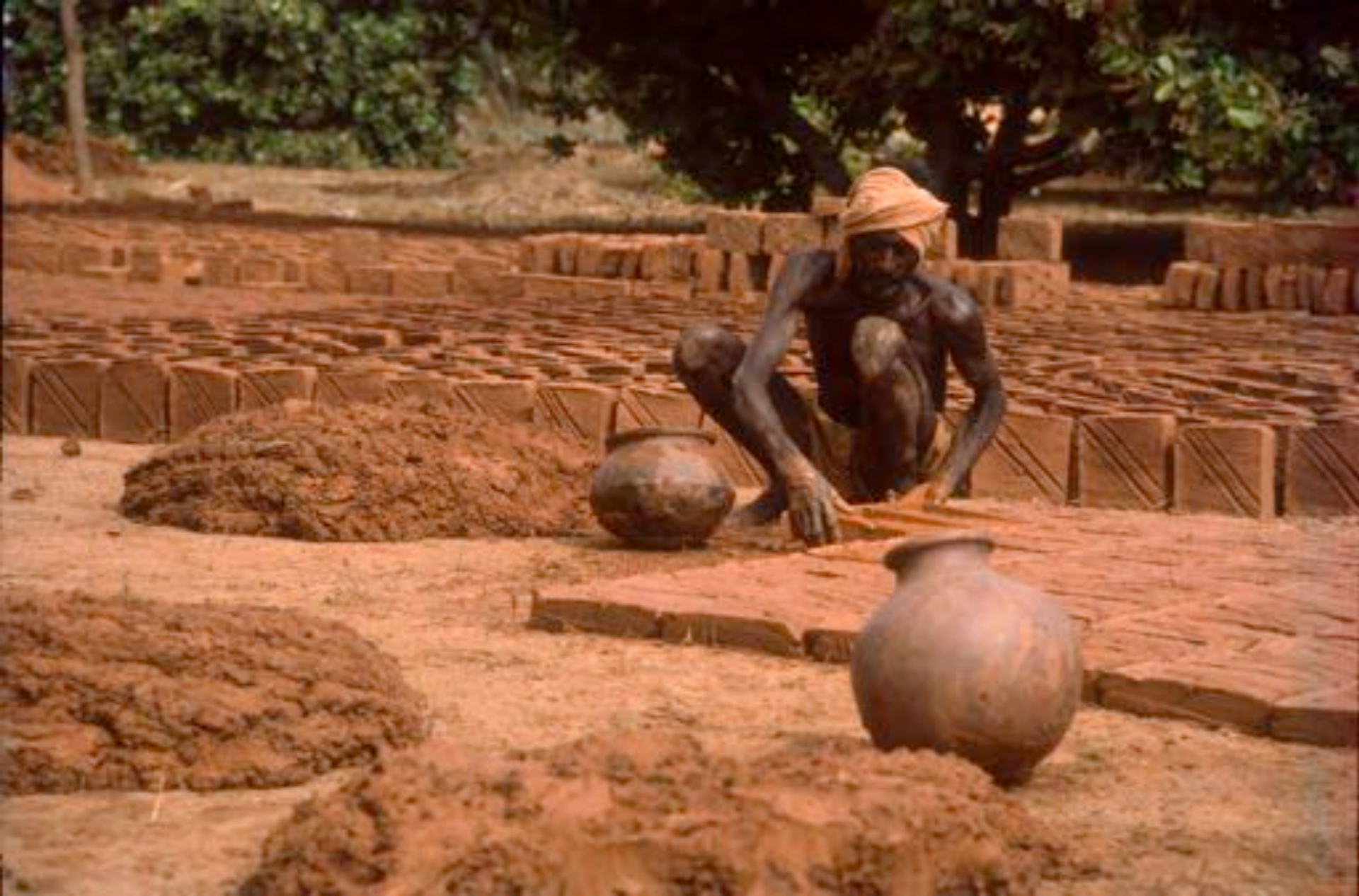
Structural bricks were made on-site with a mixture of site clay, a very sandy laterite, and clay from brick fields 20 kms away. These are vault bricks, 25 x 15 x 5 cms.
